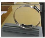
4. Wrap the clip around the post, close, and tighten back up as shown:
